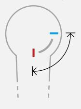
The optimal lever position for energy-efficient warm water is in the middle and allows an intuitive correct operation (ideal using temperatures 35 °C, 38 °C or maximum 45 °C).
